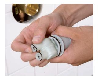
**7.** Remove the smaller O-rings from the bottom of the cylinder. Clean the openings with an old toothbrush.
