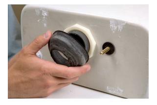
**7.** Remove the old spud washer from the threaded tail piece of the flush valve.
