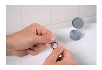
**12.** Replace the spring and rubber seat.
