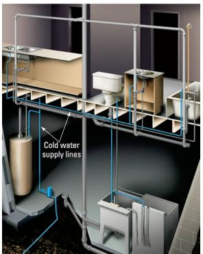
Figure 1-2: The water supply system.
